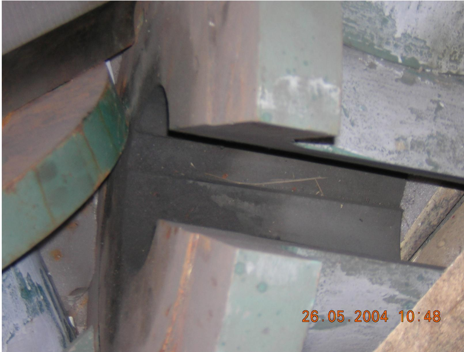
*Coupling with a sliced part has been removed for manufacturing tensile specimens*
