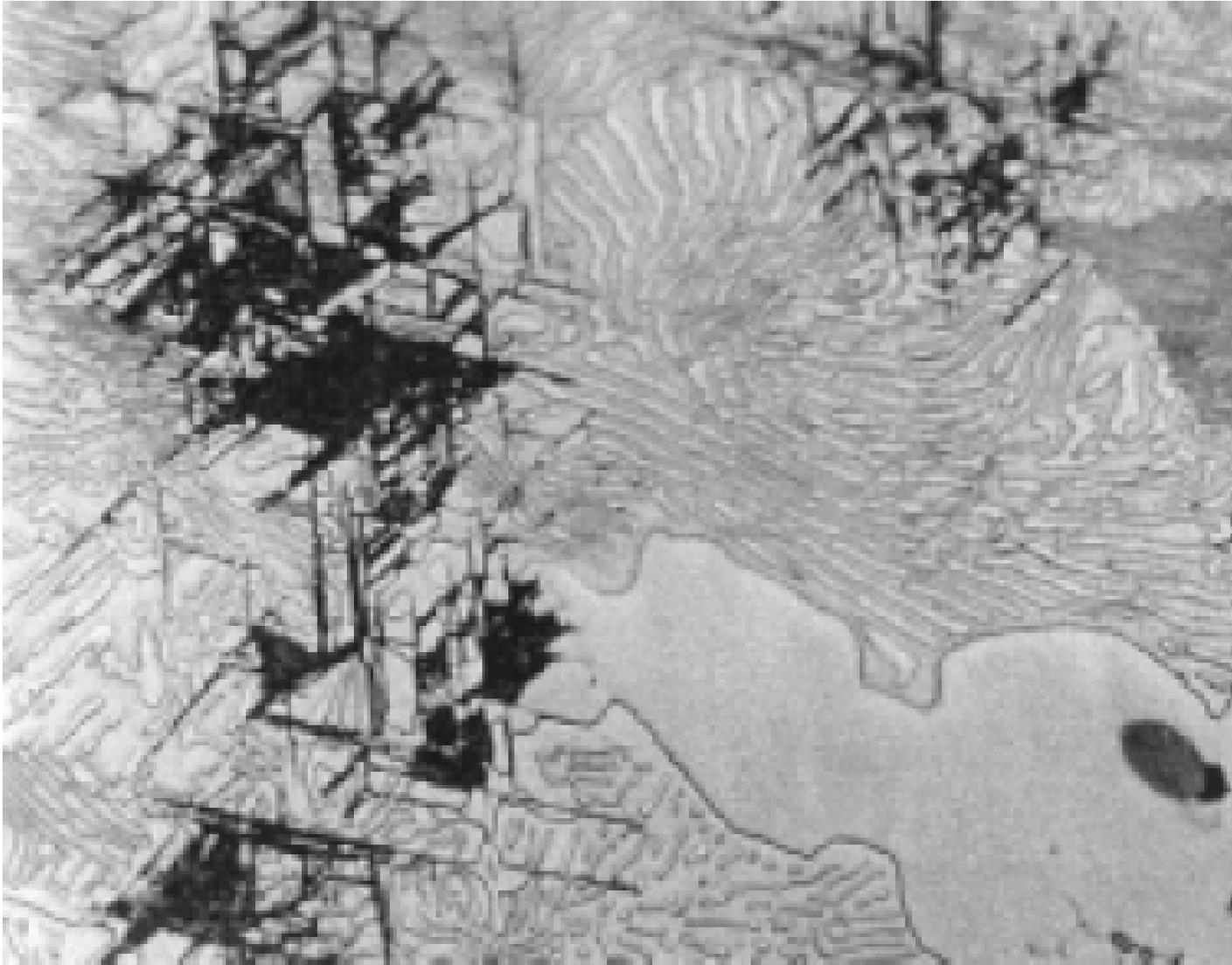
*Photomicrograph showing same area seen at lower magnification in Figs. 32 and 33 to further illustrate graphite precipitated on crystallographic planes; (1000X, nital etch).*
