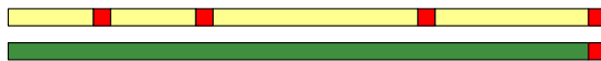
Figure 2: The cutting addition transform adds the cut size to both the items (top) and the bin (bottom)
